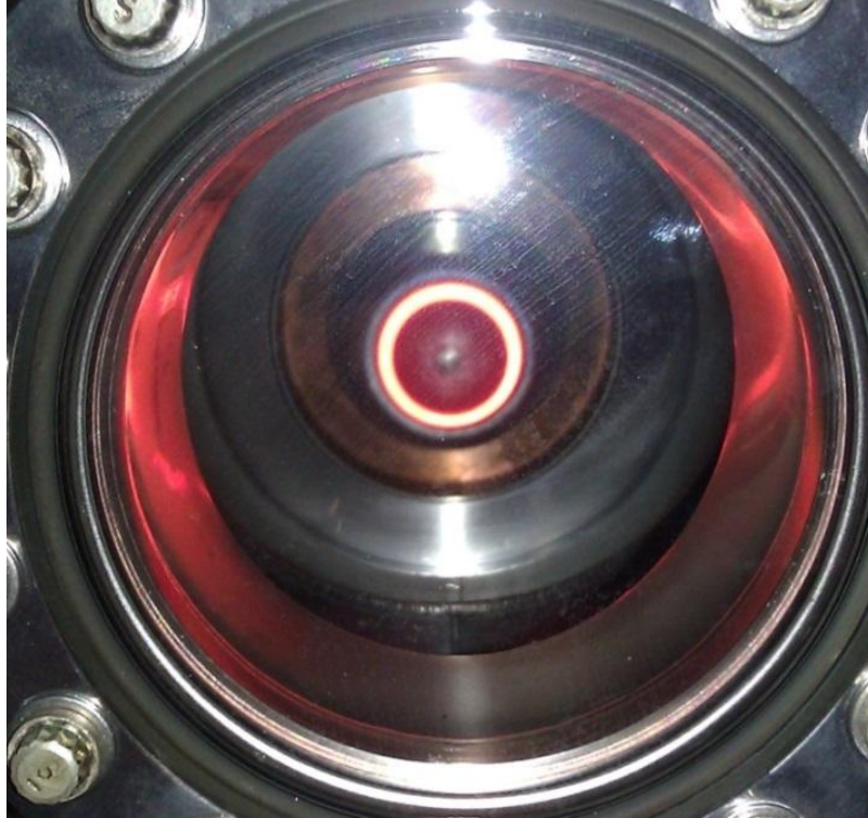
Figure 23 Emitter ring inside the testing chamber, the glowing red ring is the emitter. Electrons are emitted from the emitter surface.
