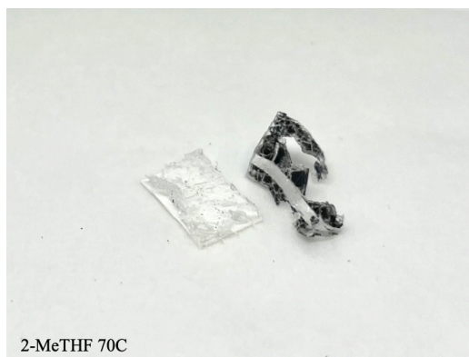
Figure 25. Solar panel fragments following 2-MeTHF treatment at 70°C.
